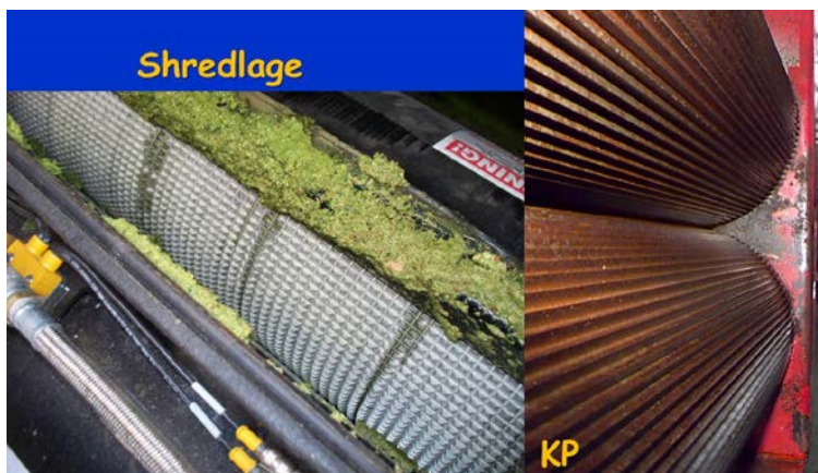
Figure 1. Roller design for Shredlage® (LHS) and Kernel Processing (RHS)
