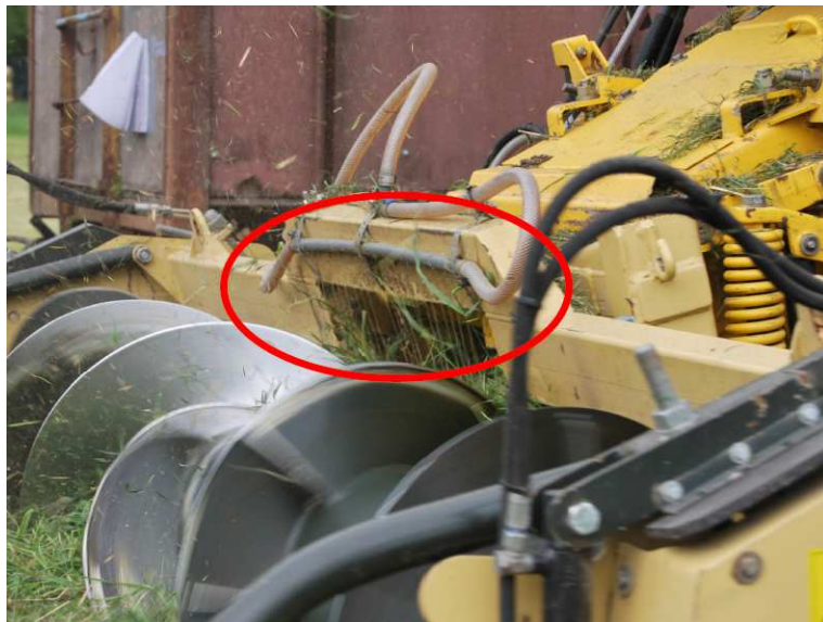
Figure 2. Jets of additive at 33 mm spacing placed at inlet channel opening
