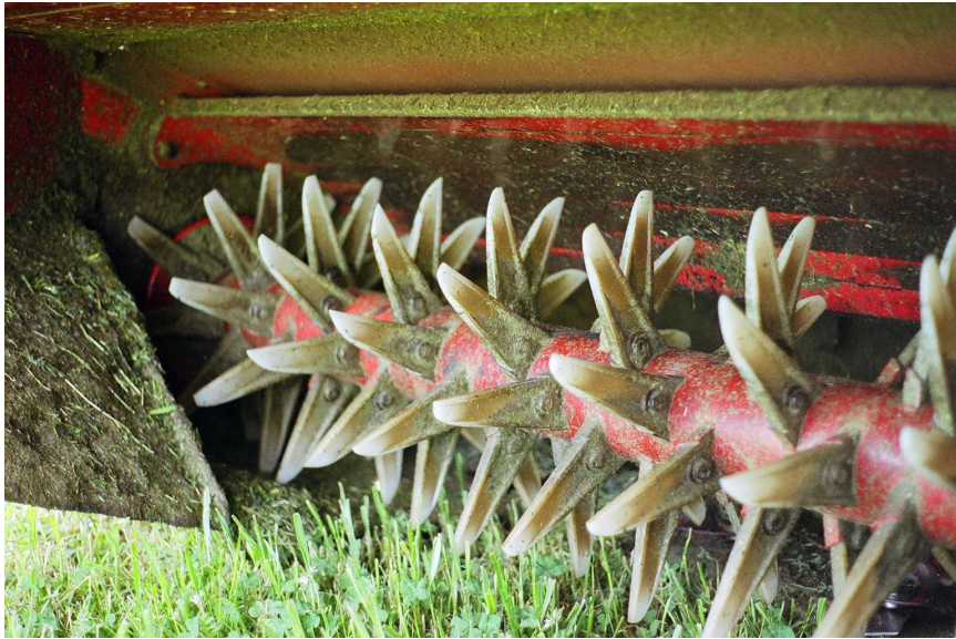
Figure 4. Tyned-type mower conditioner suitable for pastures.
