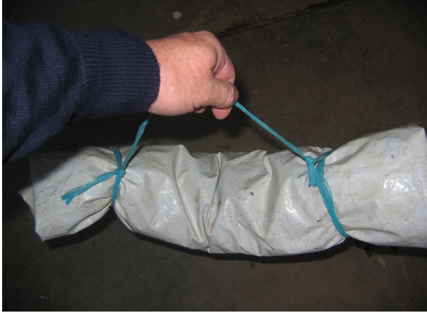
Figure 2. Sausage filled with gravel, made from waste plastic sheet
