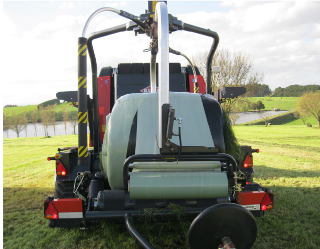
Figure 3. 3D wrapping over netwrap
