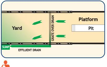
Figure 4.5: A single slope yard with drain to aid yard cleaning when a hose is used.
