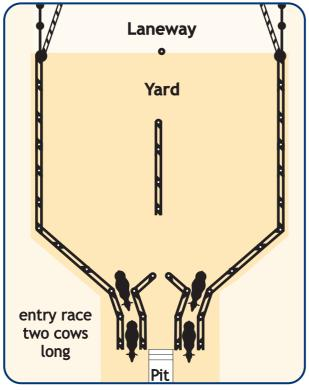
Figure 4.2: Example of a herringbone holding yard with streamlined entry into the dairy. Source: National Milk Harvesting Centre.
