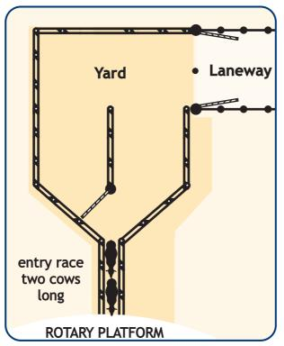
Figure 4.1: Example of a rotary holding yard with streamlined entry into the dairy. Source: National Milk Harvesting Centre.
