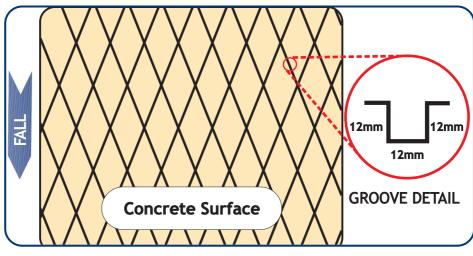
Figure 4.3: Diamond grooving for concrete surface of holding yard. Source: National Milk Harvesting Centre.
