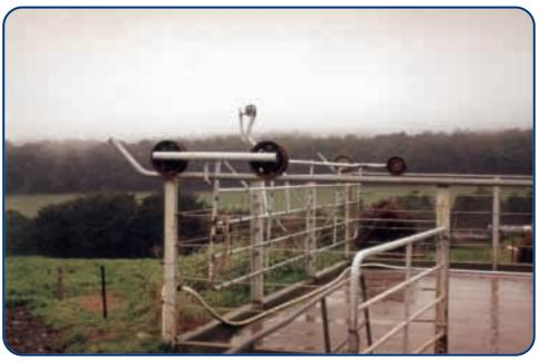
Figure 4.9: Backing gate – with anti-derail feature, but no guard for the wheels. Source: National Milk Harvesting Centre.
