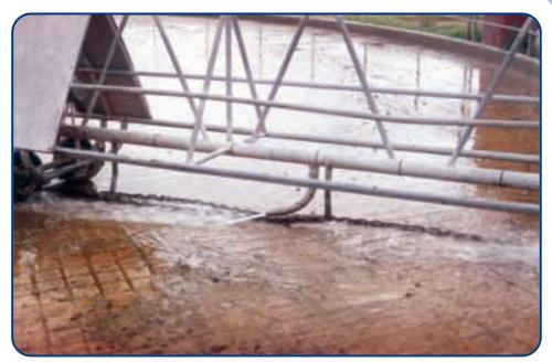
Figure 6.6: This system uses sections of chain and a number of water outlets on the backing gate.
