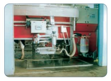
Figure 11.2: View of robotic milking system. Source: National Milk Harvesting Centre.
