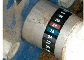
A strip thermometer attached to the milk outlet pipe.
