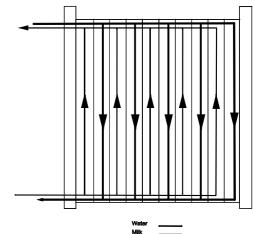
Figure 1: Single bank plate cooler (source Hakim & Schmidt)
