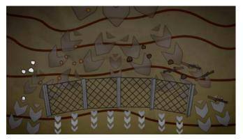
ABOVE: Ensure that the fence line curves downwards at each end so water slows and goes around the fence.
